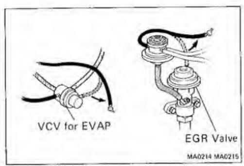
(c) Disconnect the hoses from ports of the VCV for EVAP and EGR valve, and plug the hose ends. This will shut off the EVAP purge and EGR systems.
